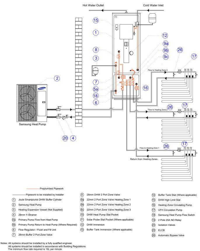
The minimum now rate required is ToL per minute The system should be power flushed for a minumum period of 1 hour to remove air.
