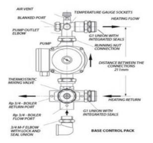
The pump module can be assembled left-, or right-handed to suit the project. The pump module is supplied unassembled, however the packaging has been designed such that components are in their relative positions for connection to the left hand side of the manifold, in an exploded view style.
