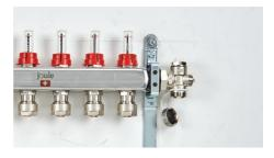
It is important to ensure the water is forced around the Underfloor Heating loops one at a time to prevent short circuiting from one manifold rail to the other. Starting at one end of the manifold, open one pipe run at a time. Open the each circuit, turn on the water supply to the top flow manifold rail and run the water until the loop is thoroughly flushed through and the water exits the lower drain point on the bottom manifold.
