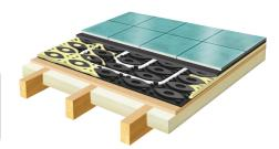
The structural plastic panel can be walked on instantly and ensures fast and efficient installation of the Inva-Heat UFH pipes by a single installer. They are suitable for all room geometries.
