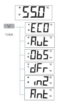
**ECO Mode:** Heating only by heat pump technology
