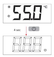
To switch off the system, hold the key for 4 seconds
