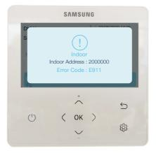
An Error code starting with "E" will appear and the power button will flash. If this happens take note of error code and contact your installer/service engineer for further assistance.
