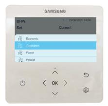
The controller is programmed to perform a legionella disinfection of the cylinder every Tuesday morning at 3am. This program will force the heat pump and immersion to heat the cylinder to 60 degrees.
