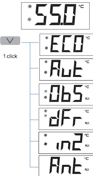
**ECO Mode:** Heating only by heat pump technology
