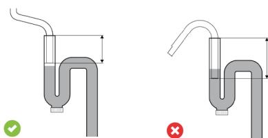
3. Make sure the drain hose is above the water level of the siphon.
